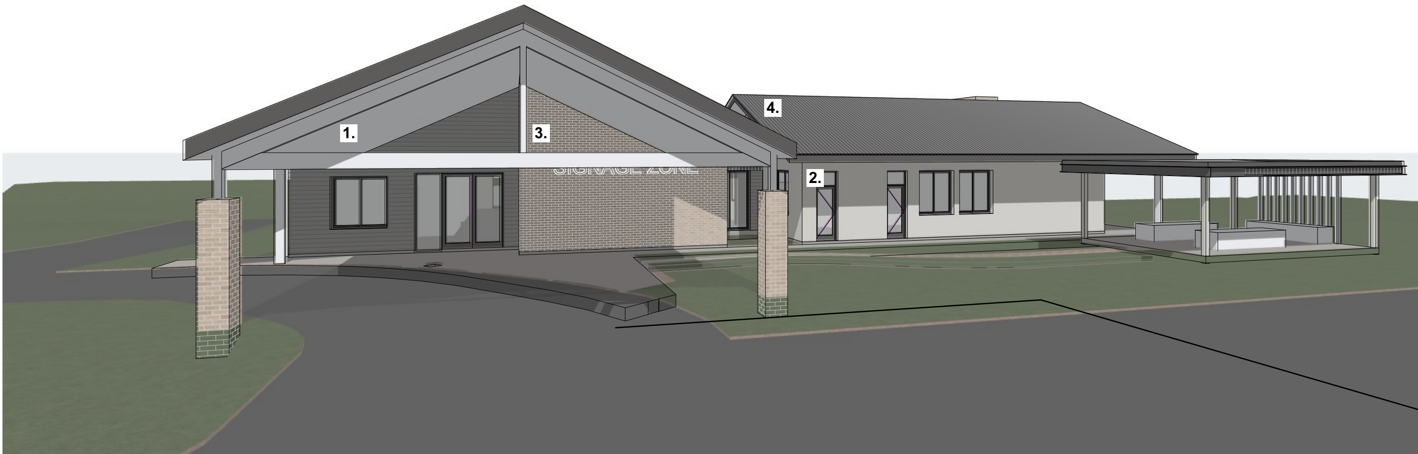
1. HORIZONTAL LIGHTWEIGHT CLADDING- WARM MID GREY PAINT FINISH
